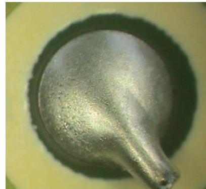
After using Shrinkage killer Solder
